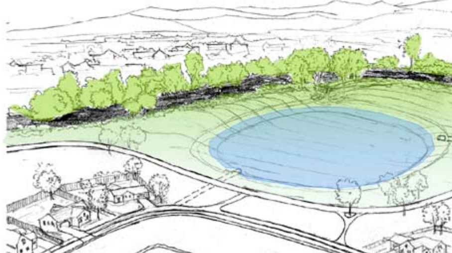
BIORETENTION PONDS FILTER WATER BEFORE IT ENTERS THE RIVER
