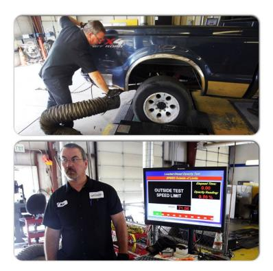
"Davis County, however, has tougher diesel tests for light-and medium-duty trucks. They use a device called a dynamometer, or "dyno" for short, which allows them to load a truck, bring it to freeway cruising speed and measure the tailpipe smoke. During its exploratory phase, the Weber-Morgan Board of Health has consulted Davis County, where they've been doing diesel emissions testing for nearly two decades." Standard Examiner, February 2015
