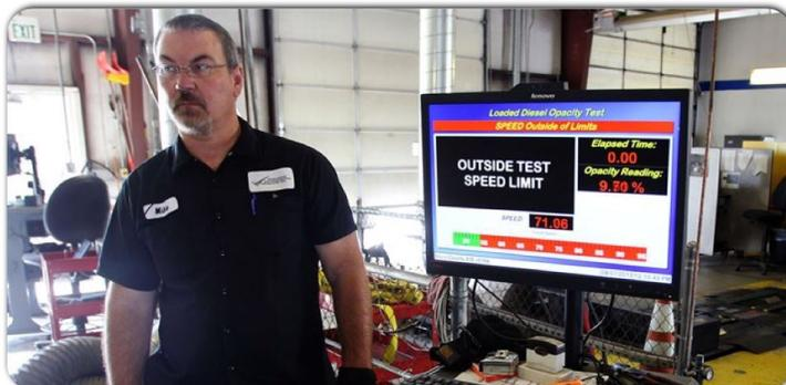
*“Davis County, however, has tougher diesel tests for light-and medium-duty trucks. They use a device called a dynamometer, or “dyno” for short, which allows them to load a truck, bring it to freeway cruising speed and measure the tailpipe smoke. During its exploratory phase, the Weber-Morgan Board of Health has consulted Davis County, where they’ve been doing diesel emissions testing for nearly two decades.”*
